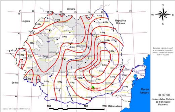
Fig. 6 P100–1/2006 design ground acceleration a_g , for an event with MRI =100 yr.
